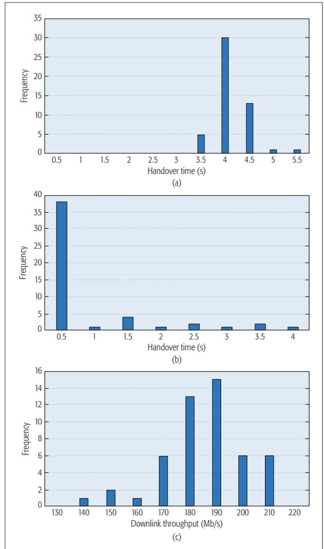
FIGURE 5. Histograms of handover times and throughputs: a) macrocell to LWA small cell; b) LWA small cell to macrocell; c) average downlink throughput during handover.
