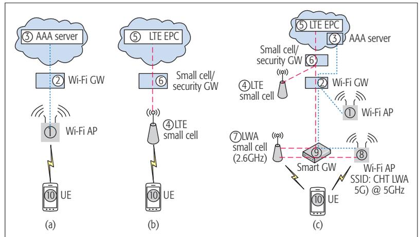
FIGURE 1. CHT's small cell network, Wi-Fi AP network, and LWA network configuration: a) WLAN network; b) LTE network; c) LWA network.
