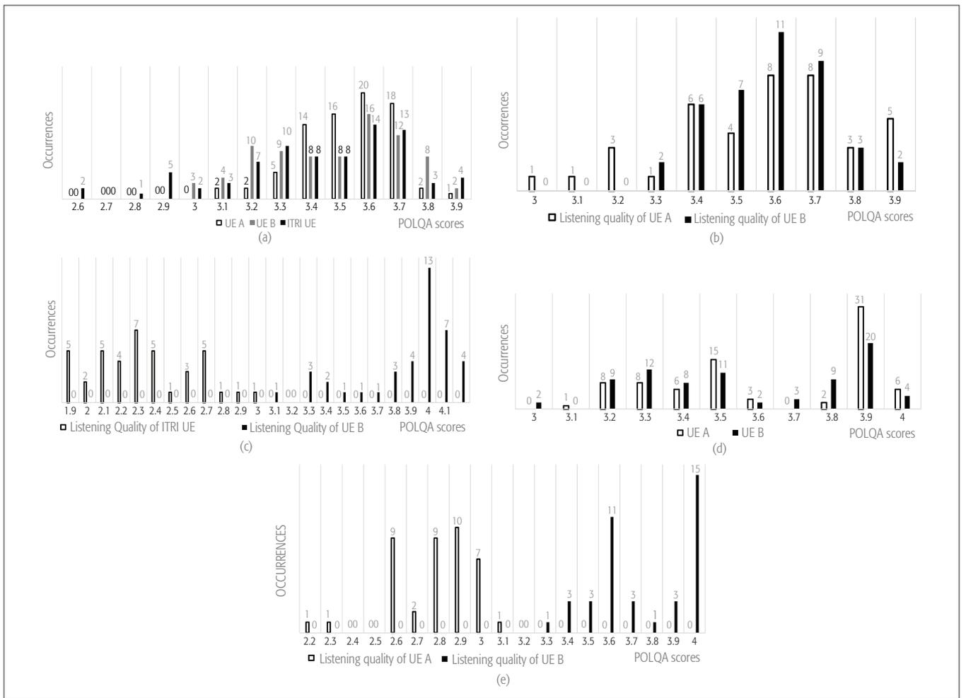
FIGURE 4. POLQA scores for eight scenarios: a) scenarios 1-3: AMR-NB between UEs; b) scenario 4: AMR-NB between UE A and UE B; c) scenario 5: AMR-NB between UE B and ITRI UE; d) scenarios 6 and 7: AMR-WB between UEs; e) scenario 8: AMR-WB between UE A and UE B.
