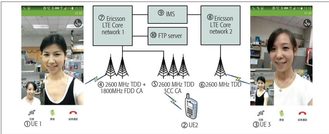
FIGURE 5. Multimode/Multiband interworking architecture.
