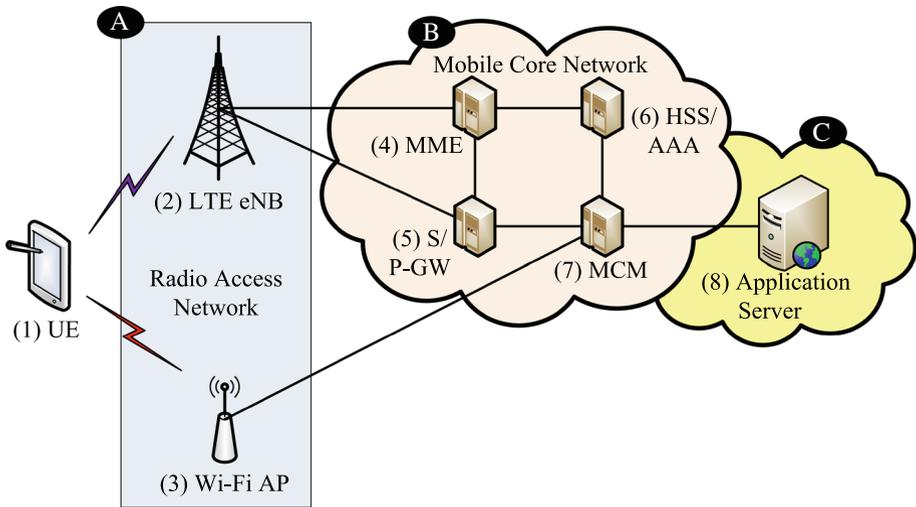
**Fig. 1** Wi-Fi and LTE integrated network architecture
