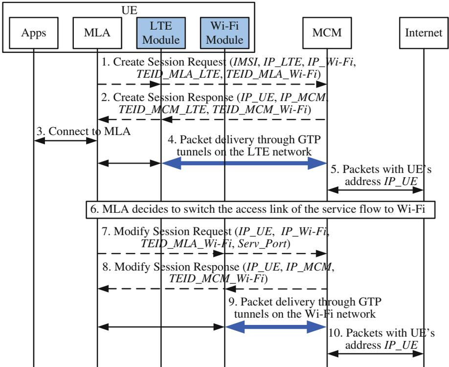
**Fig. 5** Message flow for network switching procedure
